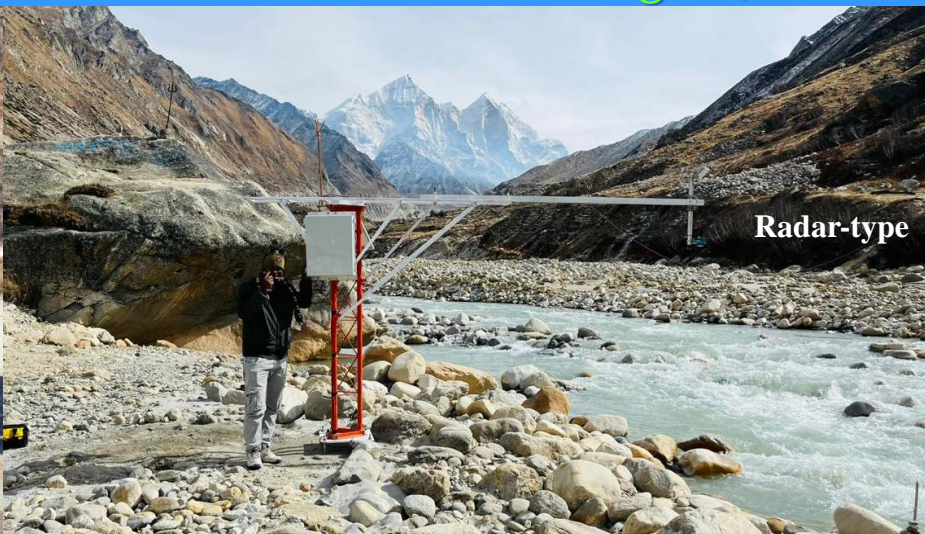
Automatic Water Level and Velocity Recorder (AWLVR)
